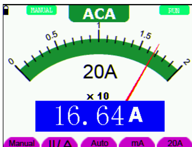
figure 30: AC Current Measurement for 20A
