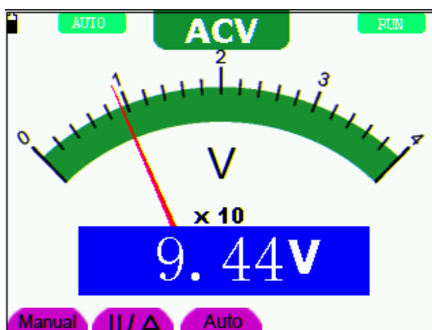
figure 26: AC Voltage Measurement
