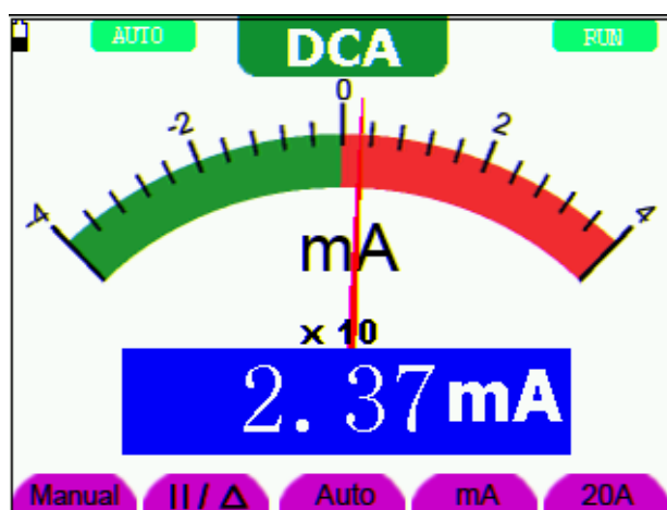
figure 27: DC Current Measurement for 400 mA
