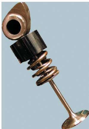
Fig.1 The cam, cam tappet, valve, and valve springs.
