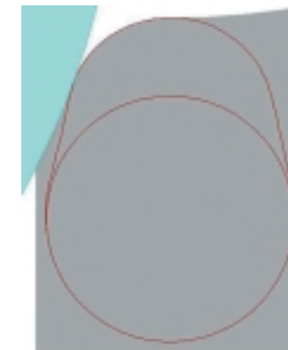
Figure 13. A snapshot from the on-screen dynamic graphics showing a finger follower cam lobe design being profiled by a cutter.
