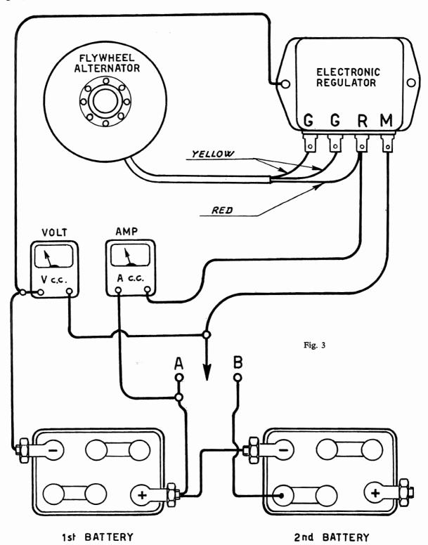
Check how works the tension regulation: install on the test bench the regulator, the pertinent alternator, the battery, the ammeter and the voltmeter, following the proper scheme.
