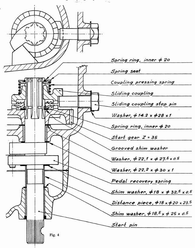
Assembly of the Flywheel-magneto, Kick-Starter and Clutch Housing (page 81)
