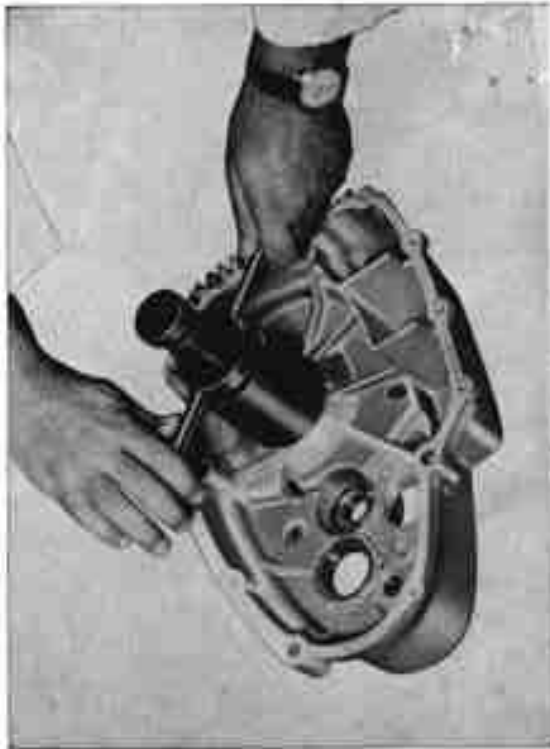
24 - Belt tensioning puller
