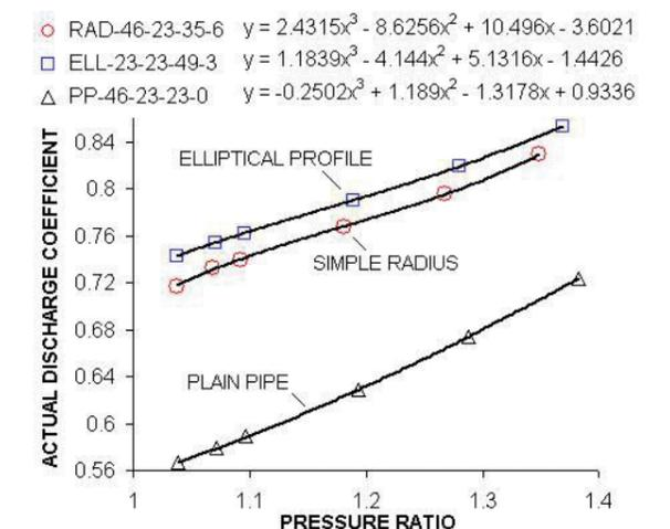
Fig.13 Curve fitted CD data for intake bellmouths
