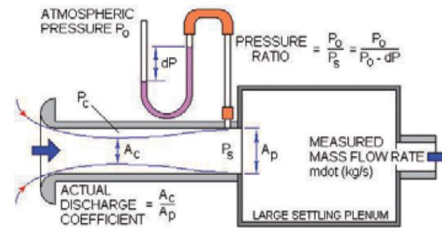
Fig.1 Measurement of Discharge Coefficients
