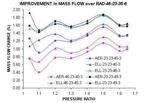
Fig.12 Airflow rate variations at intake bellmouths
