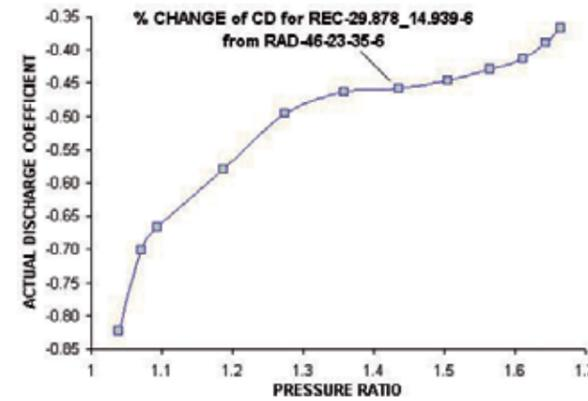
Fig.17 Loss of CD by a rectangular bellmouth
