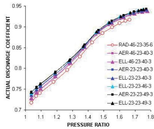
Fig.10 CD data for intake pipe bellmouths
