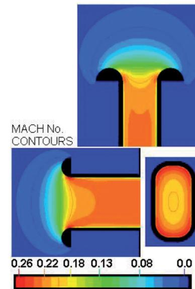
Fig.18 Velocity flow profiles at a rectangular bellmouth
