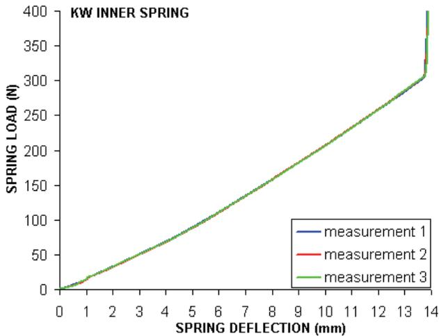
Fig.6 Three separate load measurements for a valve spring
