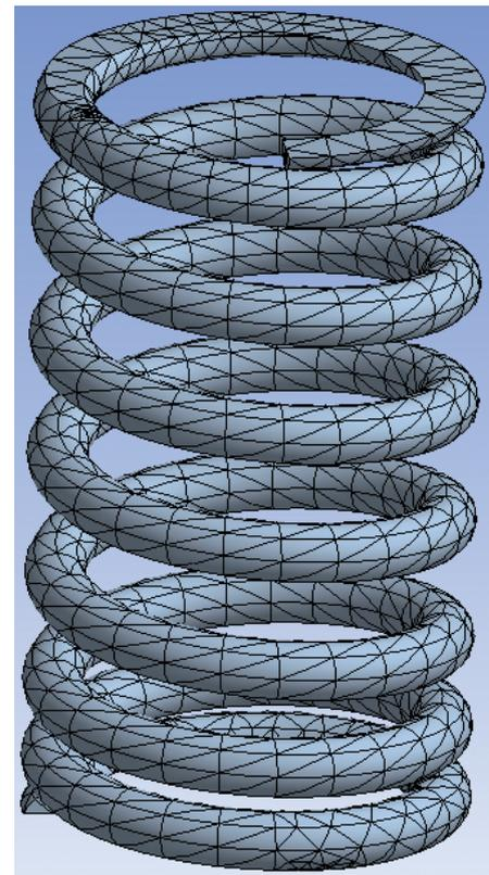
Fig.8 ANSYS FEA mesh model of the ‘KW inner’ spring
