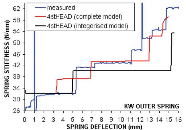
Fig.14 Measured and 4stHEAD computed stiffness of 'KW outer'
