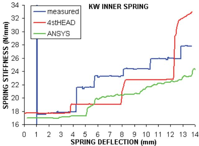
Fig.12 Measured and computed stiffness by FEA and 4stHEAD
