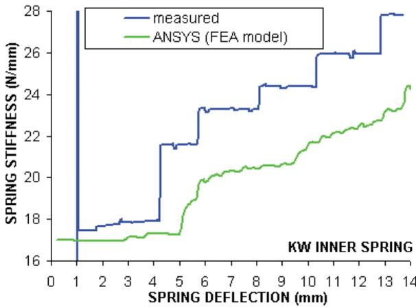
Fig.9 Measured and FEA computed stiffness of 'KW inner'
