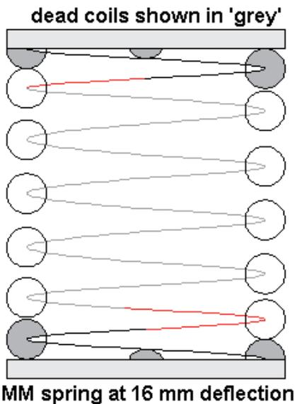
Fig.20 4stHEAD model of MM spring at 16 mm deflection
