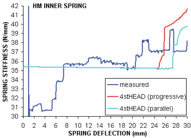
Fig.18 Measured and computed stiffness of 'HM inner' spring
