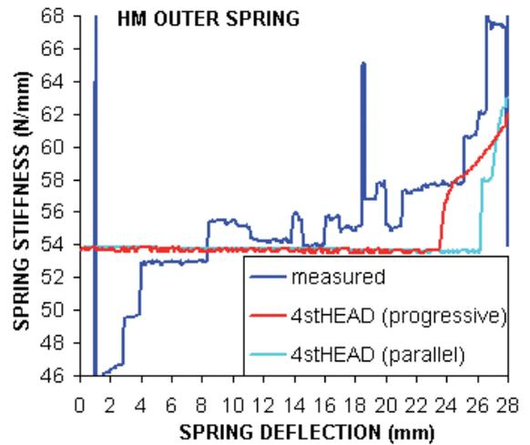
Fig.17 Measured and computed stiffness of 'HM outer' spring
