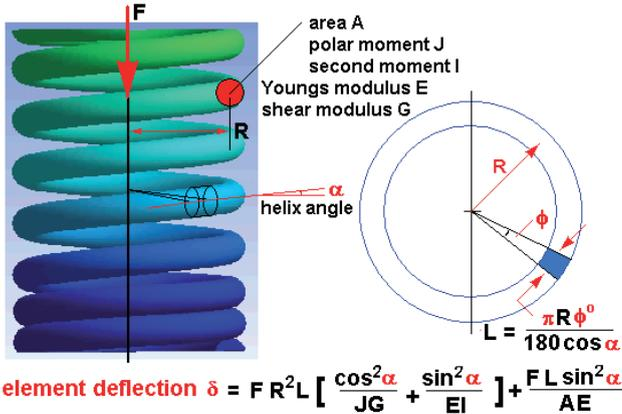
Fig.10 Model of spring deflection used in 4stHEAD
