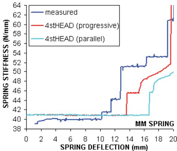
Fig.19 Measured and computed stiffness of MM spring
