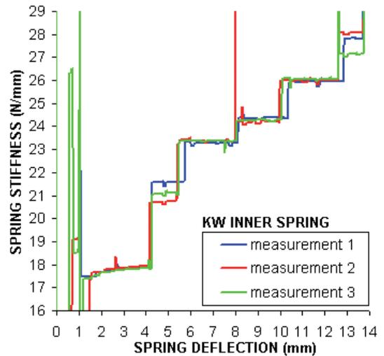
Fig.7 Three separate stiffness measurements for a valve spring
