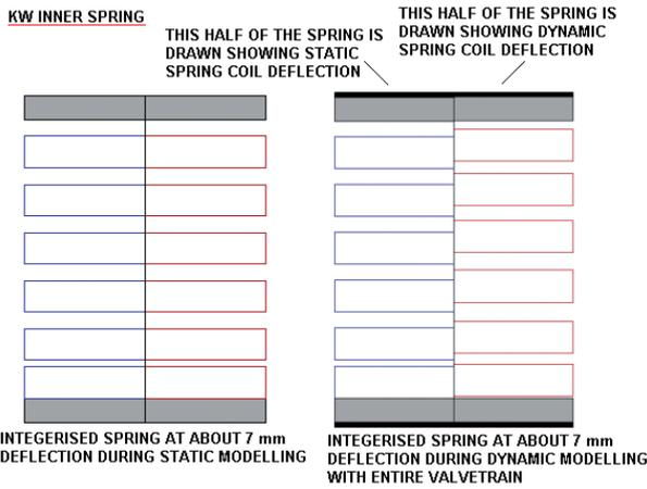
Fig.15 Static and dynamic modelling by 4stHEAD of 'KW inner'
