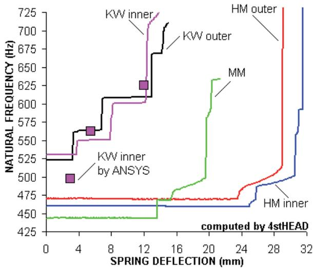
Fig.22 Natural frequencies of the five test springs
