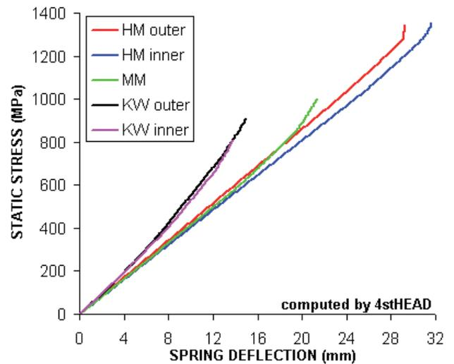
Fig.23 Stress levels for the five test springs
