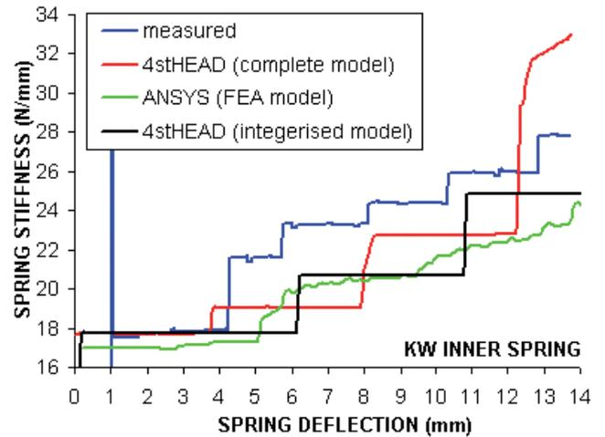
Fig.13 Stiffness modelling by FEA and both 4stHEAD models
