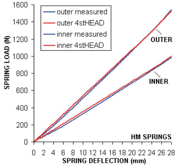
Fig.16 Measured and 4stHEAD computed loads of HM springs
