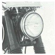
SPRINT SS DETACHABLE LIGHTS — Easy-off headlight and taillight convert any SS to a scrambles track model in minutes.
